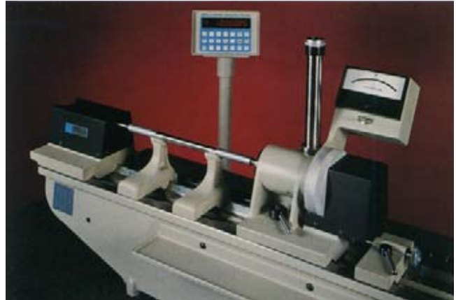
Verifying a Precision end measure length
